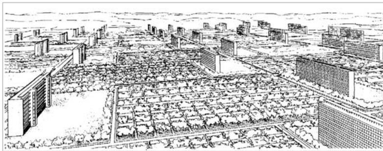
Figure 6: Ludwig Hilberseimer: Scheme for a "Mischbebauung" with L-shaped single-family houses and high-rise buildings, all oriented toward south (Hilberseimer 1931c).
